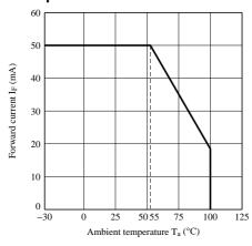
Fig.2 Diode Power Dissipation vs. Ambient Temperature
